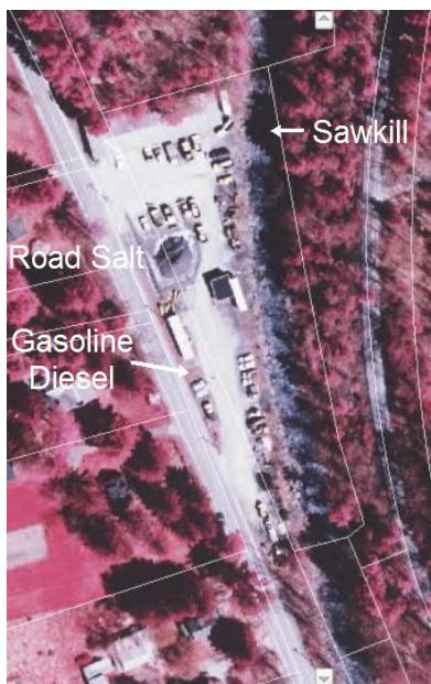
The old highway garage was a significant threat to the Sawkill. Road salt was stored as an uncovered pile, the town's gasoline and Diesel storage tanks were on-site, and the site was subject to possible flooding. There was a high risk of environmental contamination of the Sawkill. The old building was a wreck, in a state of disrepair, without adequate facilities for the employees.
